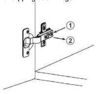
2.Attach the door back to the unit. Line the hinge up with the base plate (1), and push the back of the hinge until it clicks into place (2).
