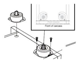
2.Gently push the legs into the leg tops, ensuring a snug secure fit.
