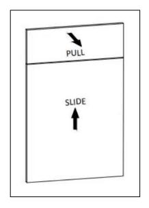
To gain access to the WC the panels are connected using Ke-Ku clips. These are removed as shown
