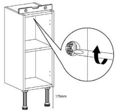
6. Screw the adjustable foot so it sits securely on the floor.
