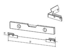
5.Gently lift the unit onto the wall brackets. Make sure the unit is level and plumb, turning the bottom screw on the cabinet hanger to adjust the height of the unit.
