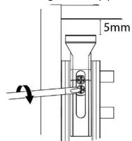
3. Measure a distance 'D' between the internal edges of the end panels of the unit and attach the wall brackets as shown below.
